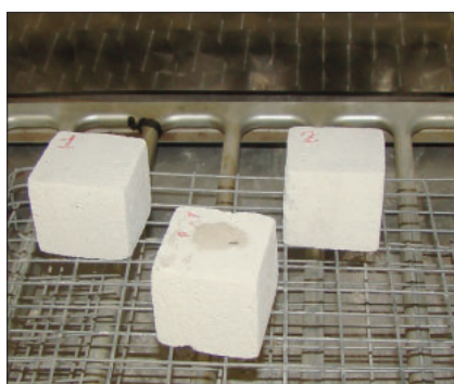
Fig. 7. Compressive strength test of gypsum foam samples according to GOST 10180
